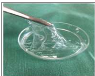
Fig. 3. The gross view of cross-linked hyaluronic acid using BDDE at the concentration of 0.8% [49]
