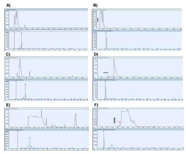
**Fig. 6.** Total ion chromatogram (TIC) of A) alcoholic beverages, B) alcoholic beverages + methanol (1%), C) herbal distillate, D) herbal distillate + methanol (1%), E) hand sanitizer, and F) hand sanitizer + methanol (1%). The red arrow indicates the methanol peak.
