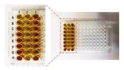
**Fig. 4.** The microplate view of samples after the complete setup of the method. 1: A to H show standards. 2: A to H shows the samples diluted (l: 20) with distilled water. 3: A to H shows the samples containing 1% methanol.
