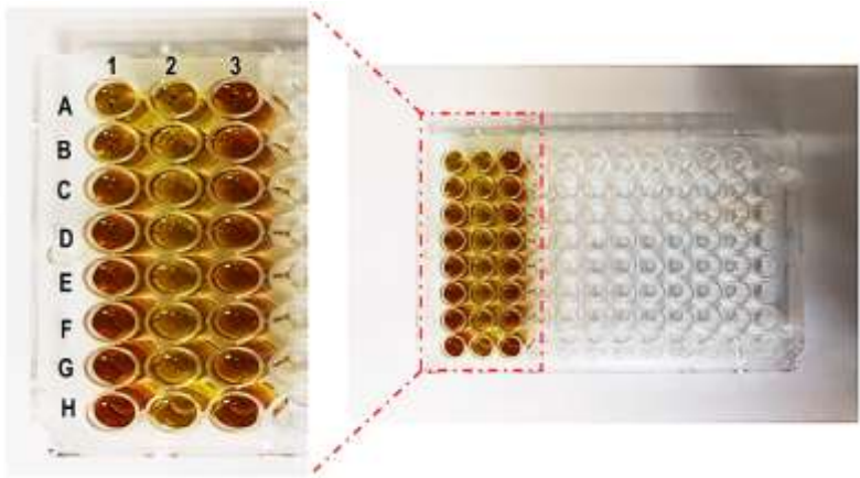
Fig. 4. The microplate view of samples after the complete setup of the method. 1: A to H show standards. 2: A to H shows the samples diluted (1: 20) with distilled water. 3: A to H shows the samples containing 1% methanol.
