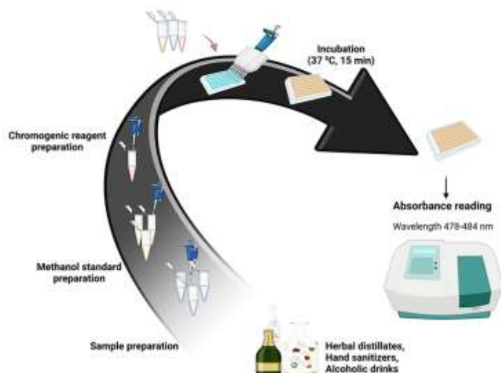
Fig. 2. Schematic illustration of the designed method to estimate the methanol amounts in alcoholic and non-alcoholic solutions.
